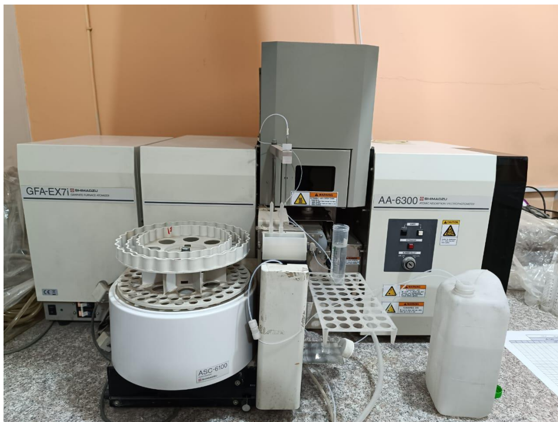
Fig. 2.3. Graphite (furnace) atomic absorption instruments the used in the measurement of the concentrations of elements.
